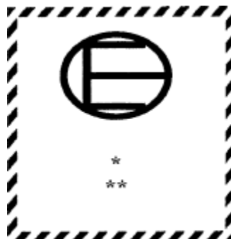
Figure A19.1. Excepted Quantity Package Marking
